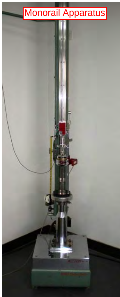
Penetration test apparatus with adjustable base
